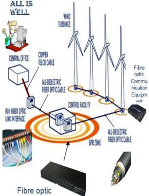
Fig.6 Typical Fibre Optic Network in Onshore Wind Farm Source:
